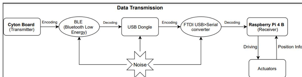
Figure 2: Data transmission flowchart between EEG and exoskeleton
